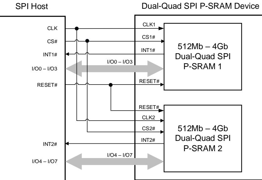
**Figure 4: Dual-CS# System Block Diagram**
