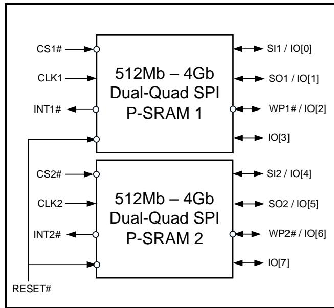
**Figure 3: Single CS# System Block Diagram**
