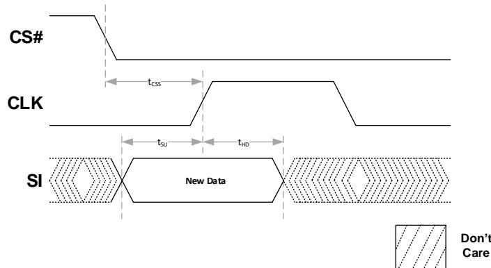
**Table 43: SDR Command, Address, XIP, and Data Input Operation & Timing**
