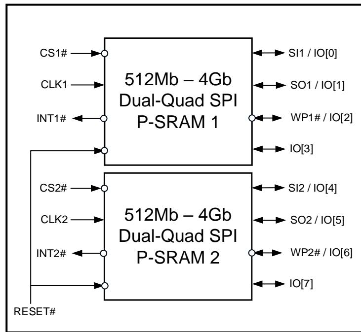
**Figure 3: Single CS# System Block Diagram**
