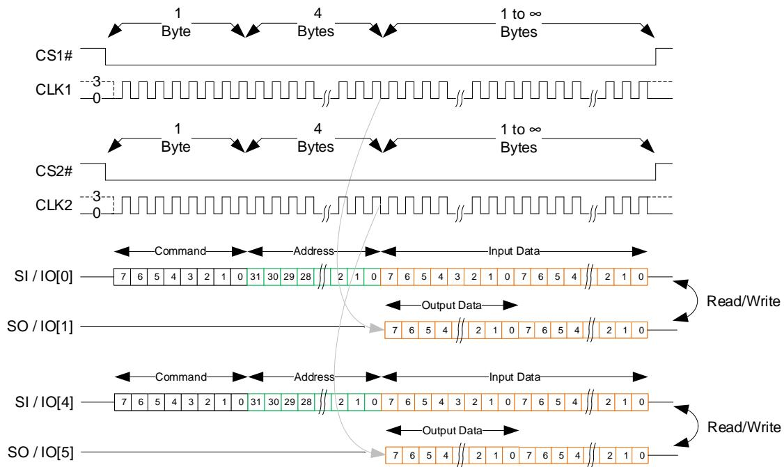
**Figure 16: Description of (1-1-1) Instruction Type (Without XIP)**
