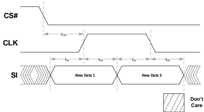
**Table 44: DDR Command, Address, XIP, and Data Input Operation & Timing**
